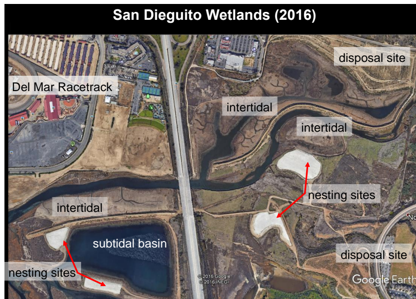
Figure 3.0.4b. During construction, the ruderal areas, old agricultural fields, and the WWII airfield were excavated and graded to create the planned intertidal and subtidal wetland habitats of the restoration project visible in this 2016 image. Image Source: Google Earth; NEGI.
