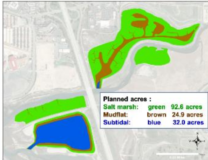
Figure 5.1.2.1. Areas of planned salt marsh (green), mudflat (brown), and subtidal (blue) habitats as provided in the Final Plan for the restoration project.
