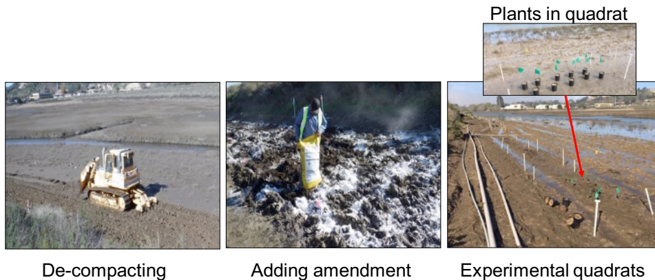
Figure 7.2.7. Images showing a tractor de-compacting soil to a depth of approximately 1.5 feet, the manual addition of soil amendments (gypsum, commercial fertilizer), and the arrangement of experimental quadrats and plants within each quadrat in the IDAPS experiment.
