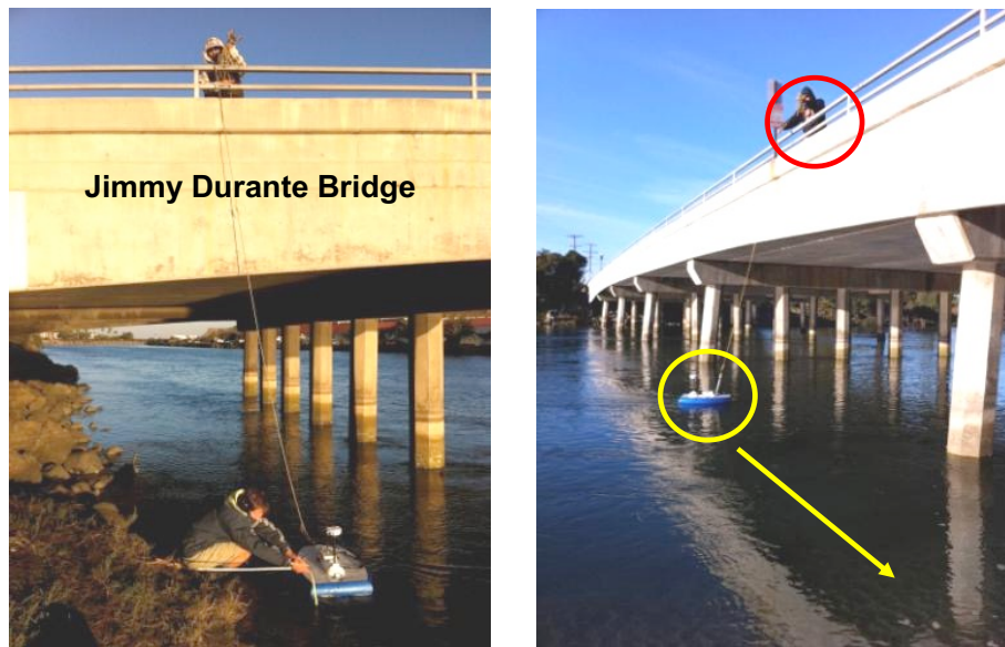
Figure 5.1.1.1. Measurements of tidal flows are taken at Jimmy Durante Bridge (0.9 km from the inlet) using a portable Acoustic Doppler Profiler/discharge measurement system (yellow circle) that is towed back and forth (indicated by the yellow arrow) across the width of the channel by monitoring staff (red circle) every 15 minutes during an incoming tide.
