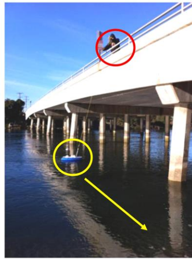
River Surveyor--Acoustic Doppler Current Profiler (ADCP)
