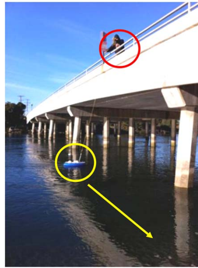
River Surveyor--Acoustic Doppler Current Profiler (ADCP)
