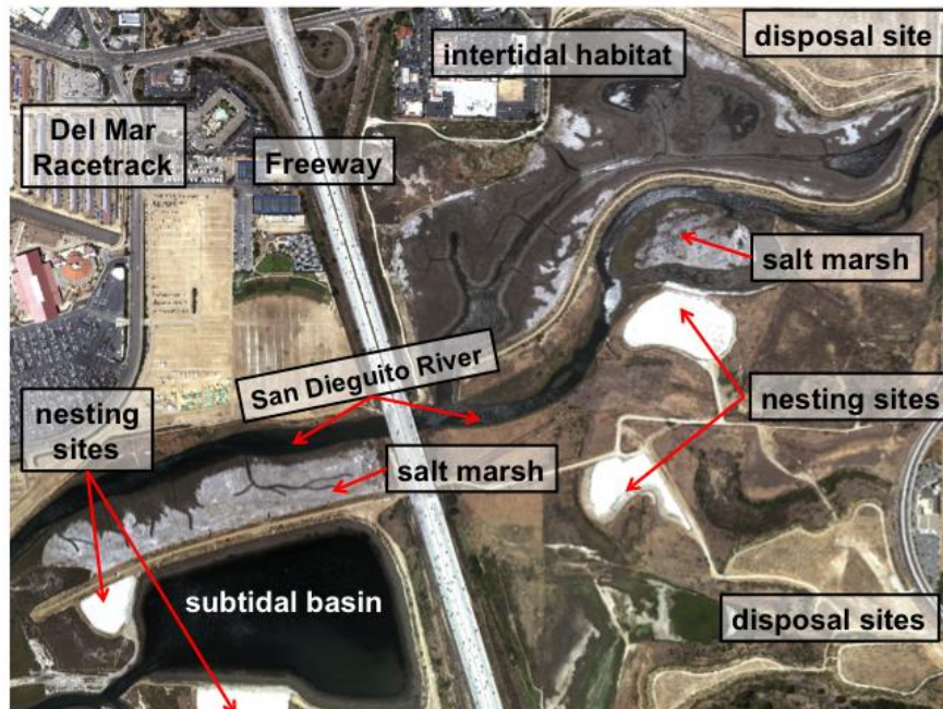
Figure 3.1.3b. During construction, the ruderal areas and old agricultural fields were excavated and graded to create the planned intertidal and subtidal wetland habitats of the restoration project.
