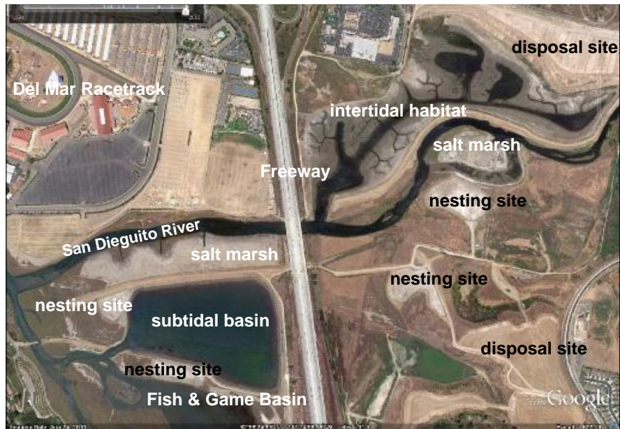
Figure 3.1.3b. During construction, the ruderal areas and old agricultural fields were excavated and graded to create the planned intertidal and subtidal wetland habitats of the restoration project.
