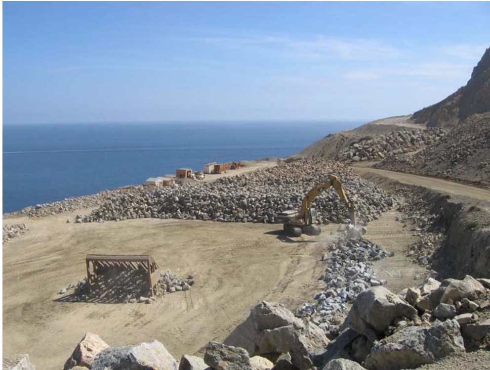
Photo G-3. Rock production at Pebble Beach Quarry. Large rocks were broken into smaller rocks by the breaker (right), and small rocks were separated out by the Grizzly (left).
