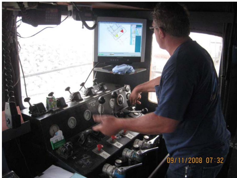
Photo G-27. Photograph taken on September 11, 2008, showing the derrick barge's anchor line control cabin and the real-time position display used to control the rock placement.
