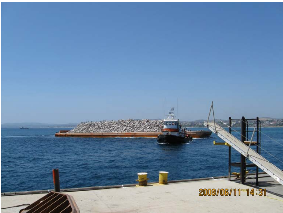
Photo C-6. Photograph showing tugboat bringing in a rock barge for tie-up with the DB Long Beach .
