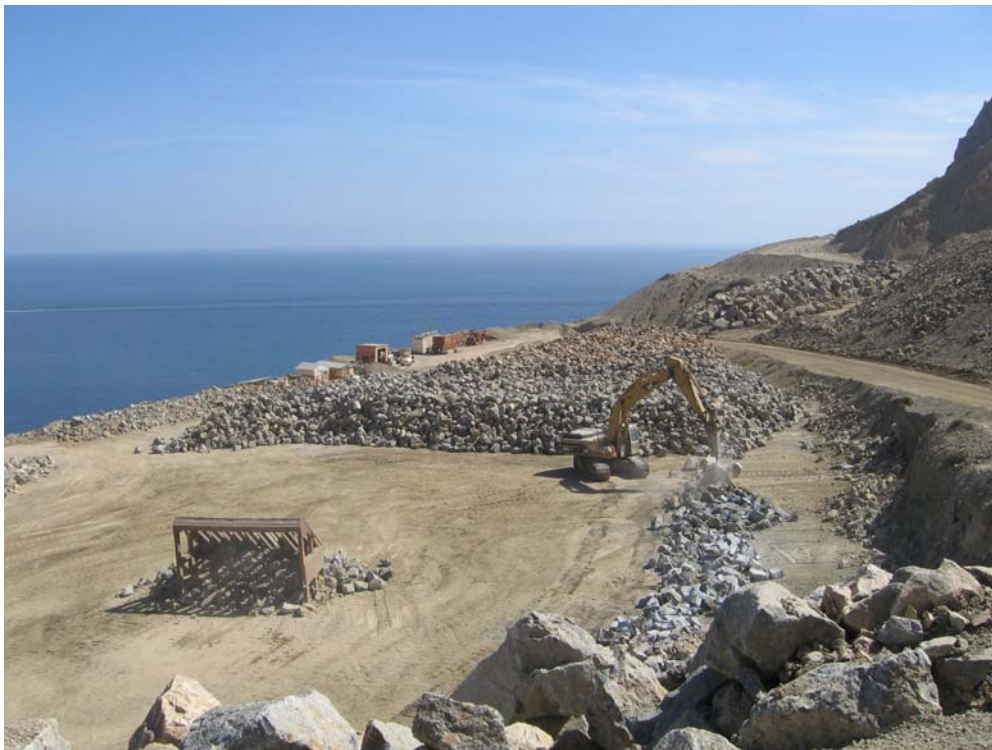
Photo C-2. Rock production at Pebbly Beach Quarry. Large rocks were broken into smaller rocks by the Breaker (right) and small rocks were separated out by the Grizzly (left).
