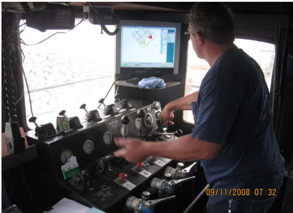
Photo C-10. Photograph showing the control room for the derrick barge winches. The derrick barge position is controlled by pulling on six, 1.5-inch-diameter wires attached to the six anchor buoys. At the right top corner is the navigation system monitor showing the location of the supply barge edge.
