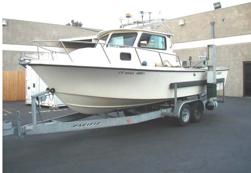
Figure 2-1. Survey boat M/V Locator, Notice Pole Mounted Reson 7101 Multibeam Sonar on the port side.
