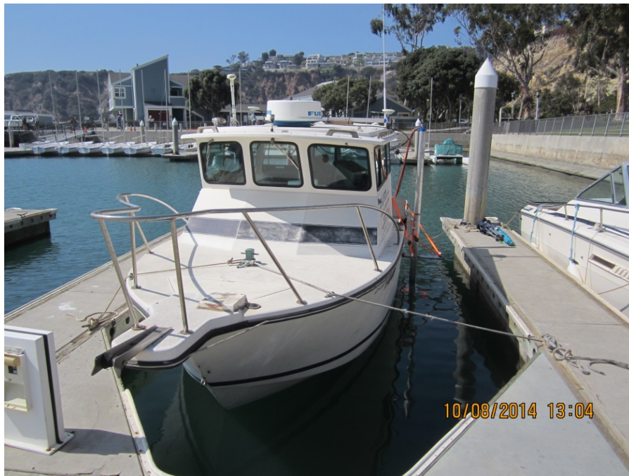
Figure 2-1. Survey boat ECO-M M/V Locator , the multibeam system is mounted on the pole at the port side.
