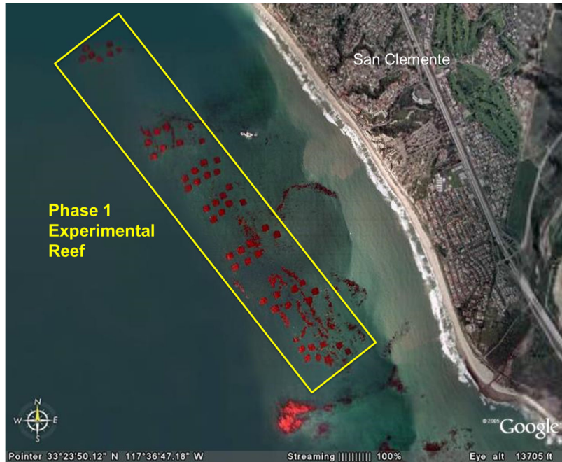
Figure 3.1.1 Infrared satellite image showing the location of the Phase 1 experimental reef (outlined in yellow) constructed for the SONGS artificial reef mitigation program. The reflectance of the giant kelp surface canopy appears as clusters of red squares, which are the locations of the 56 reef modules shown in Figure 3.1.2.
